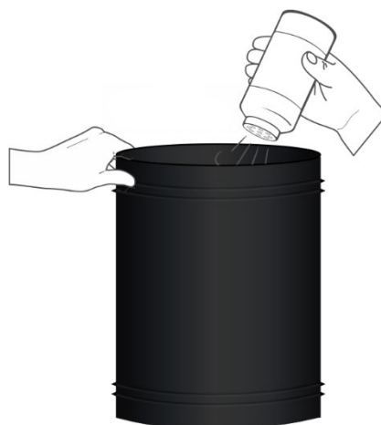
Figure 46: Powder rubber seal with talcum
