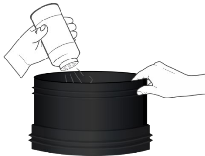
Figure 91: Powder EPDM with talcum
