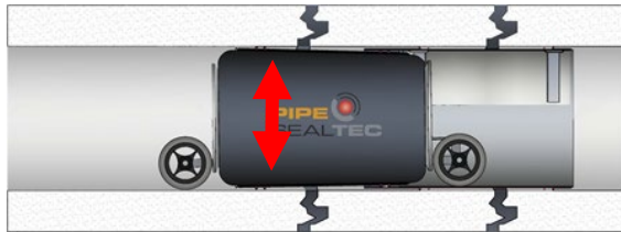
Figure 78: Expansion at the place of installation – Mounting the end sleeve
