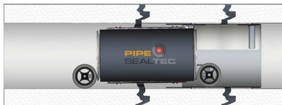
Figure 74: Mounting direction of another sleeve in a serial mounting
